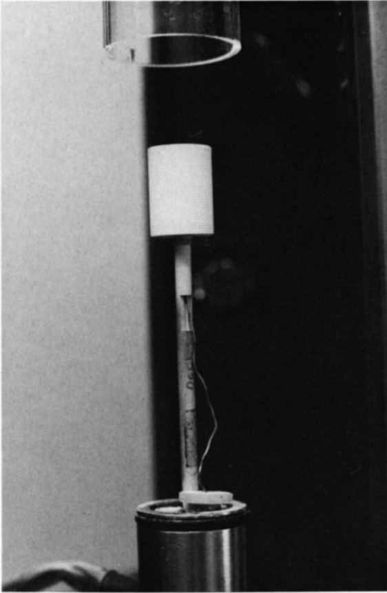
Fig. 3. TG microfurnace and TG furnace tube (above furnace) after execution of the separation procedure.
